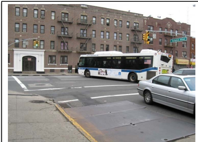
Bus stop configuration leads to turning conflicts
